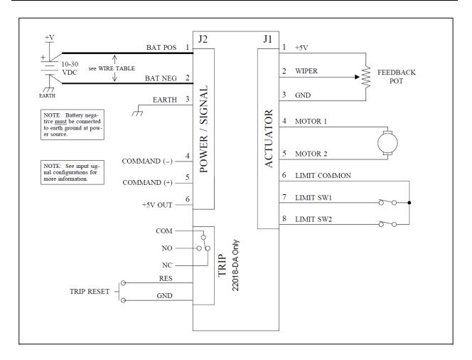
The 22018-D is rated for motors with up to 60A locked rotor or 10A running currents and has an operating voltage range from 10VDC to 30VDC. The unit is easily mounted with 2 screws and is equipped with removable screw terminals that provide for easy field wiring. The unit's size and mounting allows for an easy upgrade to a 22018-DH high resolution controller.
