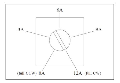
The setting should be adjusted to a comfortable level above the running current expected for the actuator and its load. When the motor current exceeds the **Trip Setting**, the motor is turned off, the yellow LED is turned on, and the form-C contact switches.
