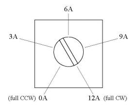
The setting should be adjusted to a comfortable level above the running current expected for the actuator and its load. When the motor current exceeds the trip setting, the motor is turned off and a fault condition is indicated (see FAULT INDICATORS).
