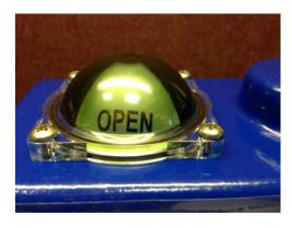
STEP 2: Remove the dome cover, dome cover O-ring, and position indicator.
